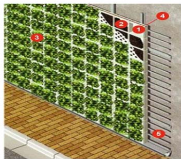
Living walls components: 1- Panels, 2- Non-soil structural growth medium, 3- Plants, 4- Remote irrigation/fertilization system, 5- Stainless steel frame, (Source: Gsky.com)
